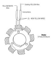
**Troubleshooting:** Engine will not start: Sometimes the source coil wires are reversed. Swap the BLUE and WHITE wires, resolder the wires and the engine should start. For OHMS testing, measure from the BLUE to WHITE. The OMS reading in the factory service manual will most likely be different than what is listed for this part. This is due to the high performance winding technology. If you have further technical questions, please refer to your service manual.
