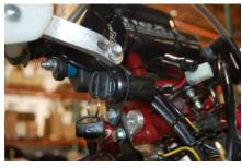
Unplug the stock 2pin & 3pin connectors underneath headlight **4**
