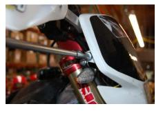
Remove upper right side clamp bolt with 10mm wrench.
