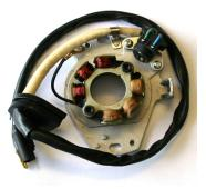
Troubleshooting: Engine will not start: Sometimes the source coil wires are reversed. You can test this by swapping out the BLUE and WHITE connections. For OHMS testing, measure from the wires as listed below. The OMS reading in the factory service manual will most likely be different than what is listed for this part. This is due to the high performance winding technology. If you have further technical questions, please refer to your service manual.
