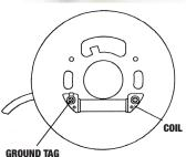
**Troubleshooting:** Engine will not start: Sometimes the source coil wires are reversed on the smaller coil. You can test this by swapping out the connections. For OHMS testing, measure from the ground tag and solder tag. The OMS reading in the factory service manual will most likely be different than what is listed for the replacement part. This is due to the high performance winding technology. If you have further technical questions, please refer to your service manual.
