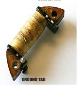
Troubleshooting: Engine will not start: Sometimes the source coil wires are reversed. You can test this by swapping out the connections. For OHMS testing, measure from the ground tag and solder tag. The OMS reading in the factory service manual will most likely be different than what is listed for this part. This is due to the high performance winding technology. If you have further technical questions, please refer to your service manual.
