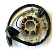
**Troubleshooting:** Engine will not start: Sometimes the source coil wires are reversed. You can test this by swapping out the BLUE and WHITE connections. For OHMS testing, measure from the wires as listed below. The OMS reading in the factory service manual will most likely be different than what is listed for this part. This is due to the high performance winding technology. If you have further technical questions, please refer to your service manual.
