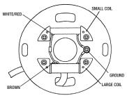
Troubleshooting: Engine will not start: For OHMS testing, measure from the ground tag and solder tag. The OMS reading in the factory service manual will most likely be different than what is listed for this part. This is due to the high performance winding technology. If you have further technical questions, please refer to your service manual.
