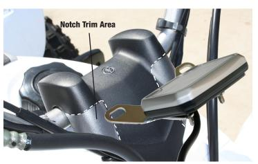
**Note:** Most ATV's have a similar type of handlebar cover. You can notch out one side at a time when pre-fitting the speedometer mounting bracket. We recommend placing masking tape on the cover and drawing your notch lines with a pen.
